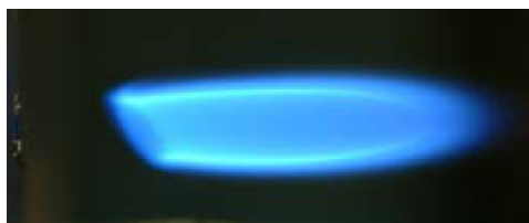
Figure 5.11: Experimental photograph of a coaxial flame, by Pablo Martínez and Jean-Marie Truffaut.
